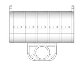
Microlift units come in a variety of sizes to fit most signage needs. Standard sizes range from 1 kilogram (2 lbs) of lift to 5 kilograms. Its important to know the types of signs and the weights before specifying Microlift units.
