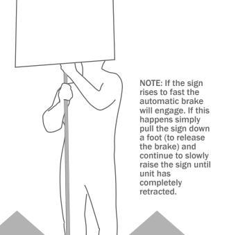
until the sign is at a comfortable working height (i.e. chest level). Release the pressure on the unit by allowing the unit to retract upwards. After a short distance the unit will lock down.
