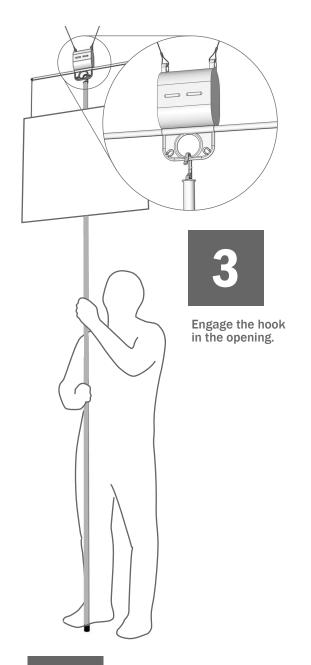
Slowly extend the pole, section by section, until the hook is level with the opening in the unit
