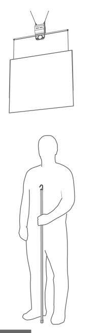
Using the Microlift pole position yourself central to the sign and slightly behind.
